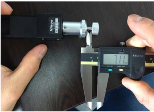
Fig. 7: Measurement by Vernier calipers
