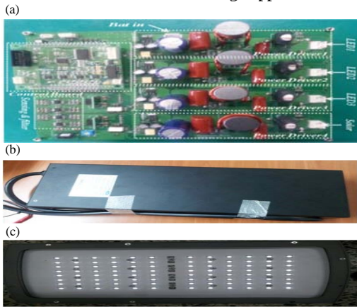
Fig. 13: Prototype circuit board; a) operation drive; b) battery system and c) 96W LED lamp
