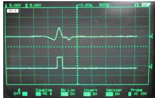
Fig. 3: Pulse generated when passing the grith weld
