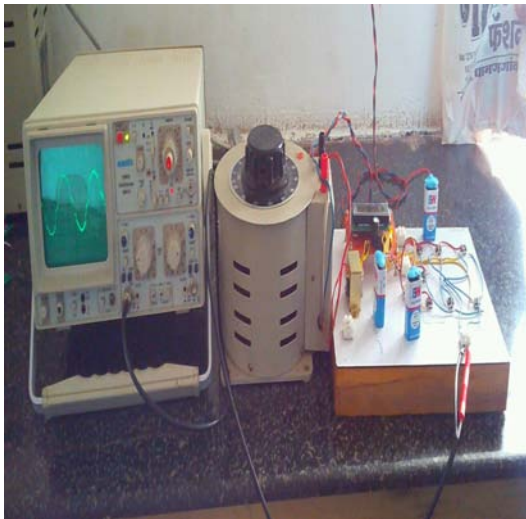
Fig. 6: Complete assembly of the experimental setup of 7-level inverter with output waveform
