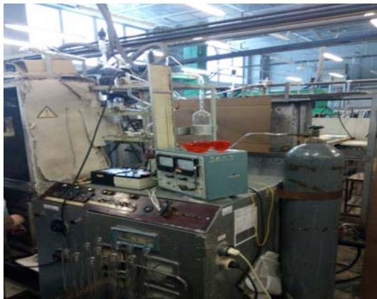
Fig. 2: Evacuating post for pumping of luminescent lamps air
