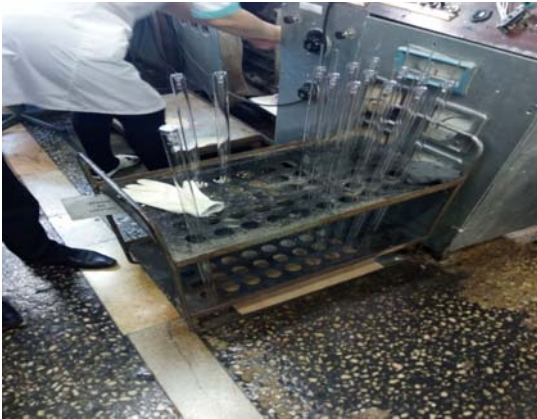
Fig. 1: Racks with evacuating lamps
