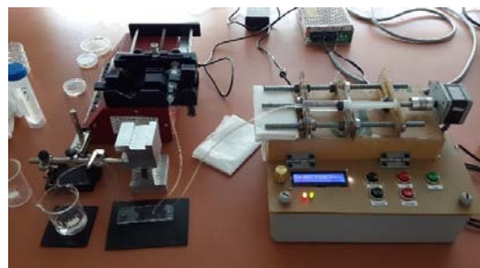
Fig. 3: The experimental setup for fabricating microbeads using the microfluidic infusion system in an ESCO class II biological safety cabinet
