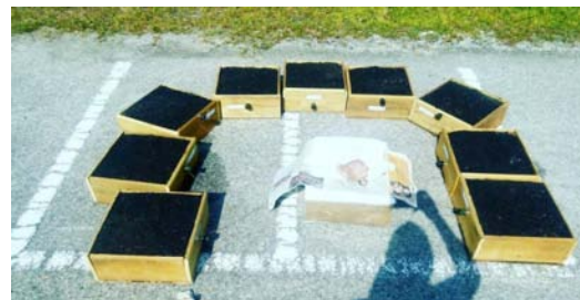
Fig. 5: Arrangement of models connected with data logger in field experiment
