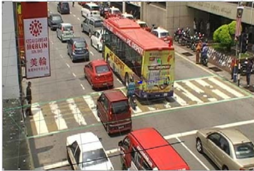
Fig. 3: The rectangular polygon drawn in accordance to the ratio of actual dimension to fit with the sequence image in scale adjusted process
