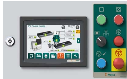
Fig. 3: Touchscreen and remote control of the cone crusher
