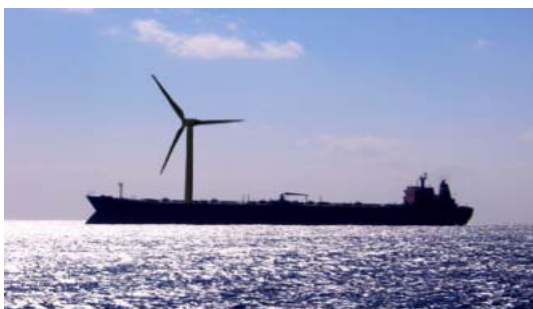
Fig. 9: A tanker ship using the conventional wind turbine
