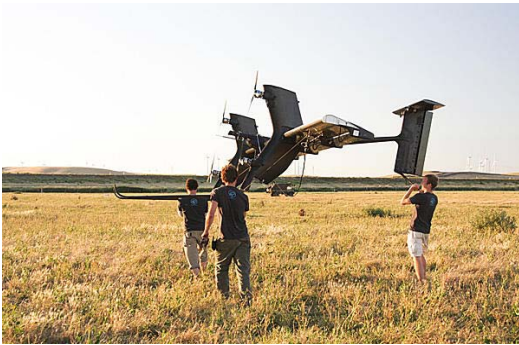
Fig. 15: The airborne wind turbine getting ready
