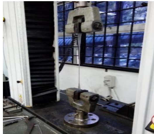
Fig. 3: Tensile test while in progress
