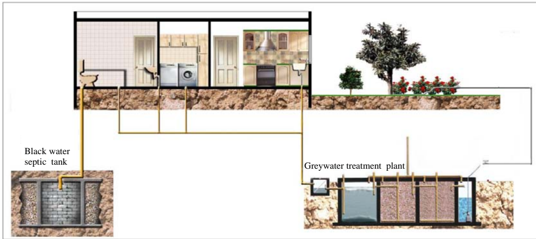
Fig. 1: A proposal for the management of rural effluents at the household level
