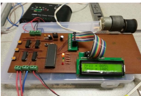
Fig. 8: Primary battery bank discharging
