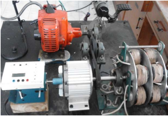
Fig. 2: Parallel hybrid electric vehicle simulator
