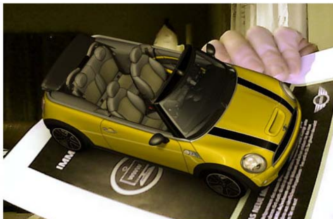
Marker transformed into ‘augmented reality’ when held in view of a webcam. Output as displayed on a computer screen
