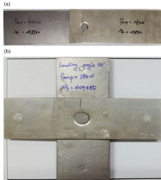
Fig. 7: Fatigue failure specimens; a) Tensile-shear and b) Cross-tension specimens
