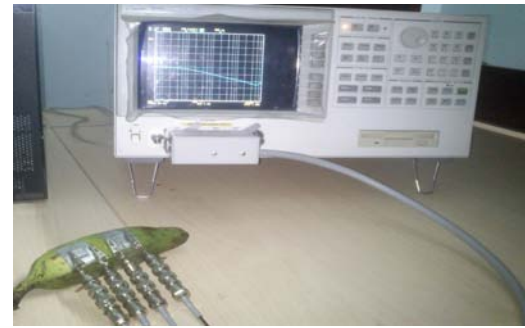
Fig. 7: Schematic of the impedance measurement with four electrode method using compound electrodes developed
