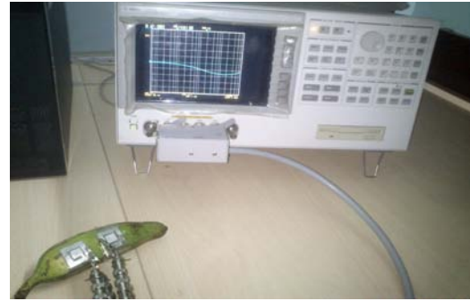
Fig. 6: Schematic of the impedance measurement with two electrode method using compound electrodes developed
