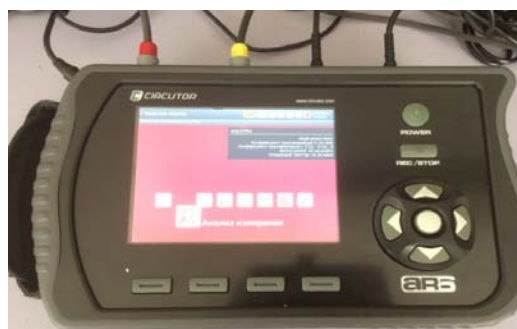
Fig. 6: Appearance and connection scheme of electrical energy quality analyzer CicutorAR6 to the unit according to the determined TPP of building objects
