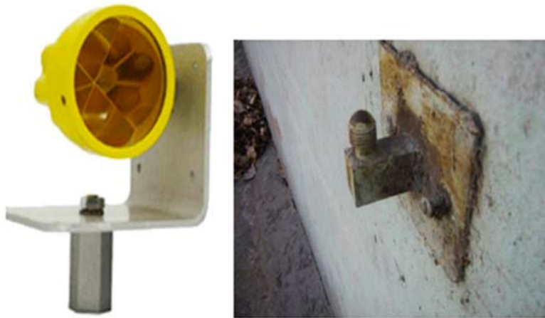
Fig. 6: Monitoring prism and sedimentary mark
