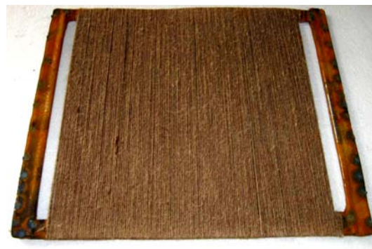
Fig. 1: Four layers of kenaf fibers woven around a steel frame
