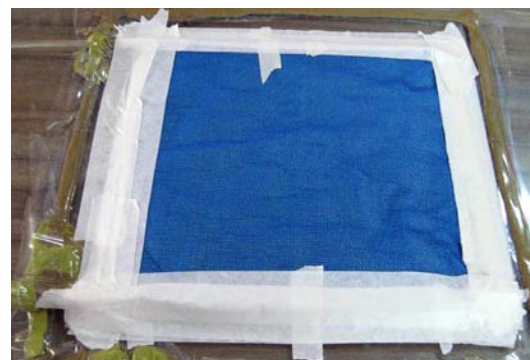
Fig. 2: The matrix in the vacuum infusion method
