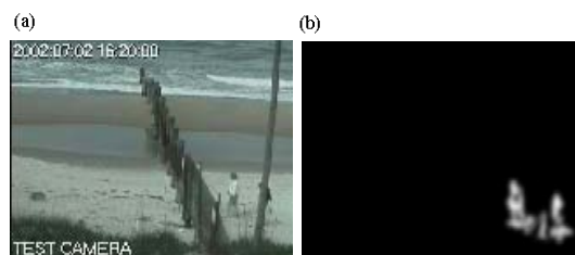
Fig. 6: Adaptive kernel density based camouflage moving object detection
