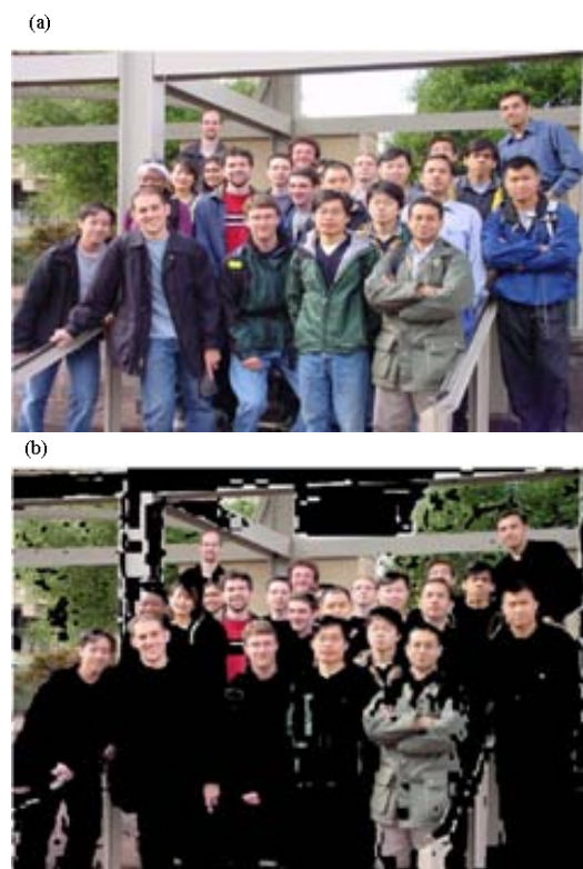
Fig. 3: a) RGB to YCbCr conversion and b) Remaining pixels after masking the lower image plane
