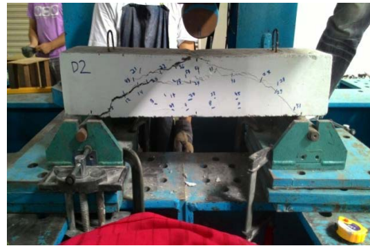
Fig. 8: Mode of failure for retrofitted sample
