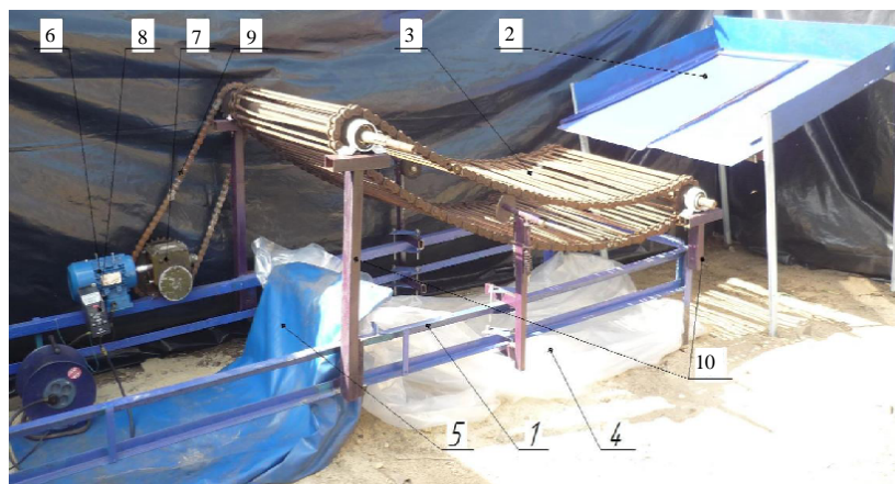
Fig. 6: General view of the laboratory equipment for studying the intensity of onion set thrashed heap[ separation: 1) Frame; 2) Container for preliminary storage of thrashed heap; 3) Separating rod elevator; 4) Canvas for collection of inclusions; 5) Canvas for separated products; 6) Electric motor; 7) Single-stage reducer; 8) Variable speed drive; 9) Chain gear and 10) Supporting rack
