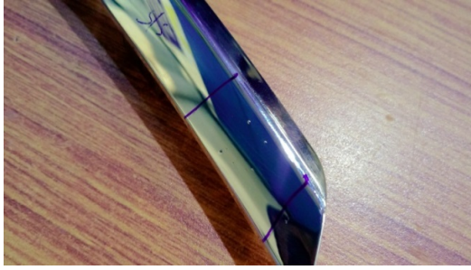
Fig. 1: Silver streaks on plated part
