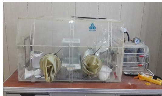
Fig. 7: Acrylic vacuum glove box
