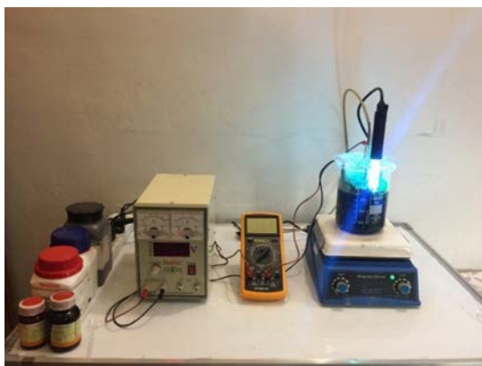
Fig. 2: Photograph of the experimental system used for batch photoelectron-fenton
