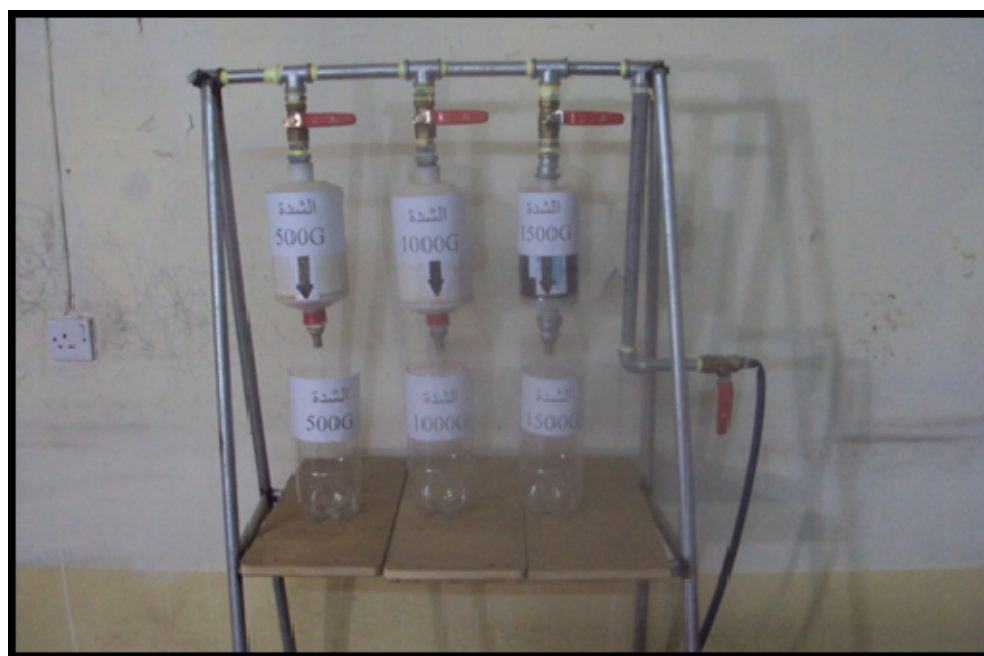
Fig. 1: Magnetic fuel treatment device for water with 500, 1000 and 1500 G
