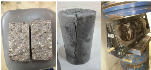
Fig. 15: The specimens after failure during the splitting tensile strength test
