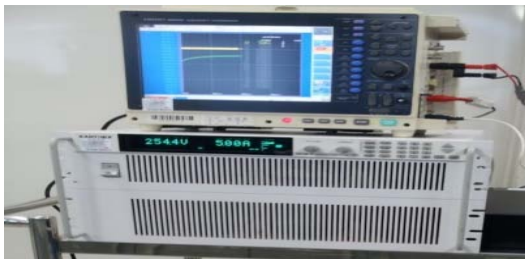
Fig. 7: A view of lithium secondary batteries battery pack (259 V/10.4 Ah) charge, discharge tests
