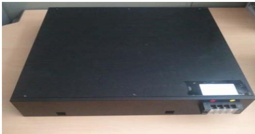
Fig. 6: Fabrication of lithium secondary battery pack (259 V/10.4 Ah)
