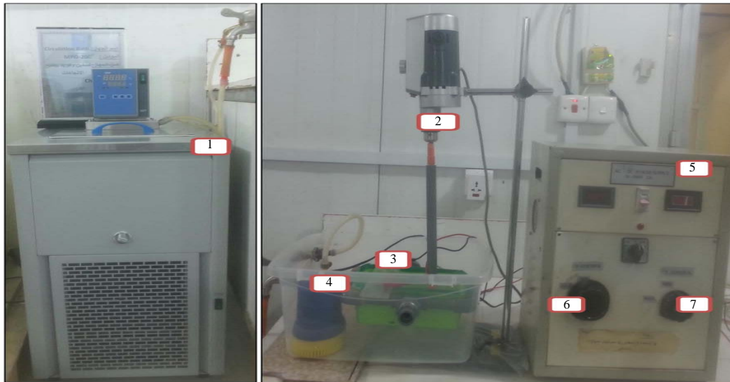
Fig. 1: Photographs of MAO coating unit: 1) Circulation bath (cooling system); 2) Mixer; 3) Coating container; 4) Cooling container; 5) Power supply; 6) Voltage gauge and 7) Current gauge
