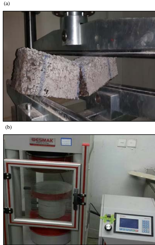
Fig. 2: Test machine and proto samples under test: a) Flexural test and b) Compression testing machine
