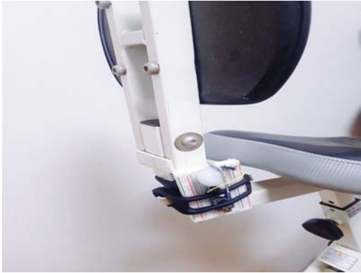
Fig. 5: Infrared sensor attached to bicycle
