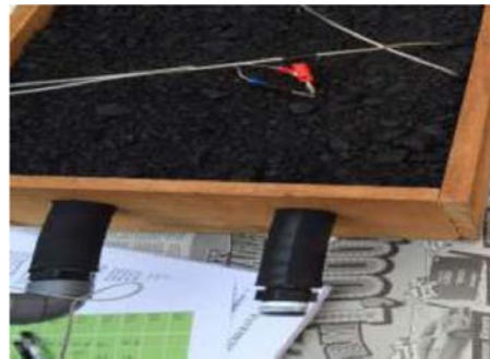
Fig. 2: Asphalt placement rubber tube embedded (a)
