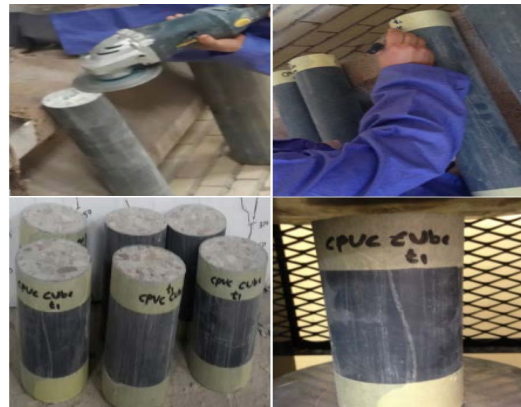
Fig. 6: Preparation of specimens to test
