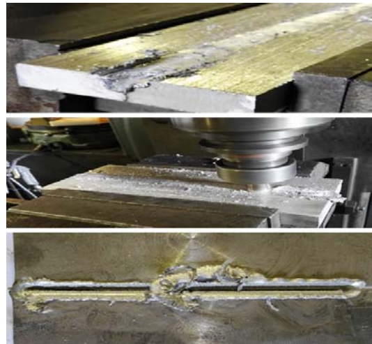
Fig. 3: FSW Plates welded in the anticlockwise direction with rotational speed of 1120 rpm in the anticlockwise and welded speed of 10, 14 and 21 mm/min
