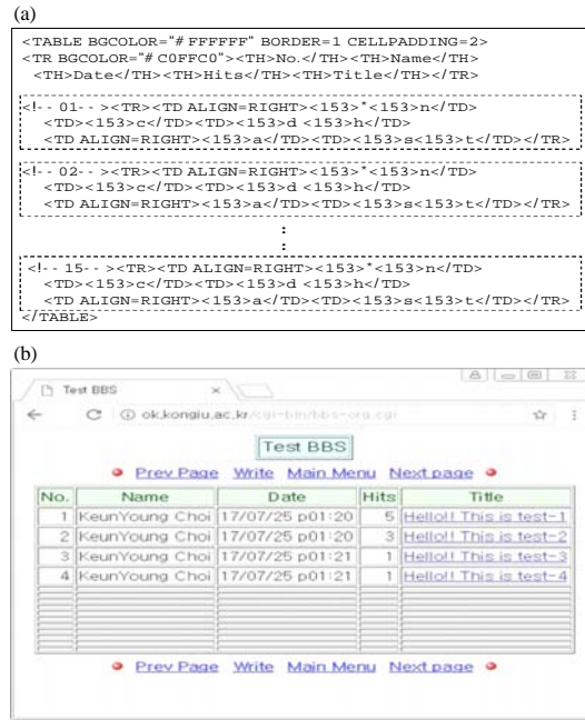
Fig. 5: Weakness example of the PSSI technique; a) Repeated part of the web-document source and b) Data ended table
