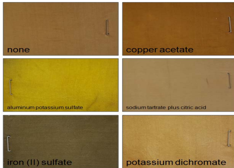
Fig. 3: Staining patterns of dye from the C. sinensis var. assamica -fermented leaf and color changes by mordants
