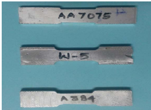
Fig. 6: The prepared specimen as per ASTM-E 606
