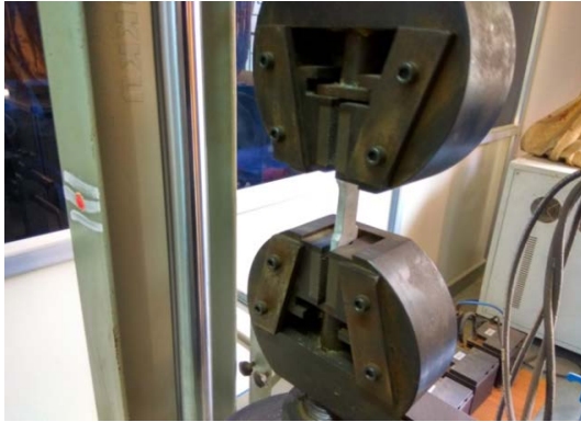
Fig. 8: Multi axial fatigue testing machine’s mechanical wedge gripper with the specimen in loaded position
