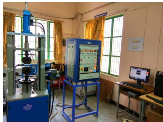
Fig. 7: Multi axial fatigue testing machine
