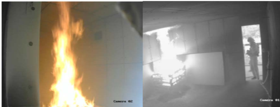
Fig. 9: Combustion of wood pallets and discharging water
