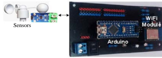
Fig. 3: Sensor components structure
