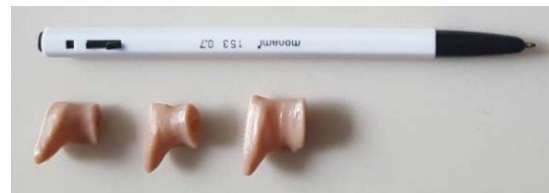
Fig. 5: Hearing aid ear shell shape manufactured by the 3D printer depending on the DICOM image thickness
