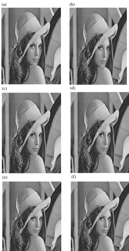
Fig. 5: Comparison of Lena image compressed and reconstructed by both algorithms; a-c) PCA algorithm at CR = 10, 70 and 90%, respectively; d-f) PCA-modified algorithm at CR = 10, 70 and 90, respectively
