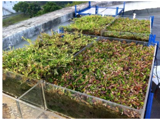
Fig. 1: Experimental green roof test beds at the rooftop level of college of engineering building, UNITEN
