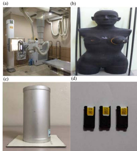
Fig. 1: X-ray equipment; a) DRS-definium; b) ART phantom; c) OSLDnanoDot and d) X-ray cylinder
