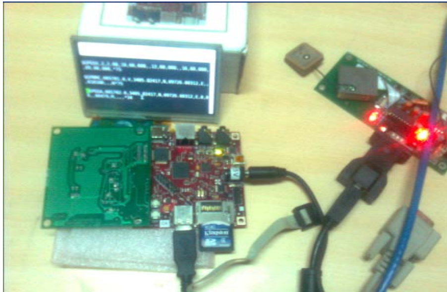
Fig. 13: GPS receiver interfacing with Beagle board
