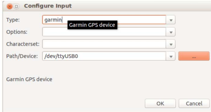
Fig. 10: USB Garmin GPS device setup
