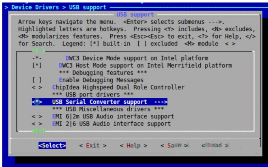
Fig. 9: USB to serial port converter support setup
