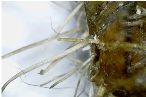
Fig. 9: Microscopic image-tear failure edge (0° fibers)
