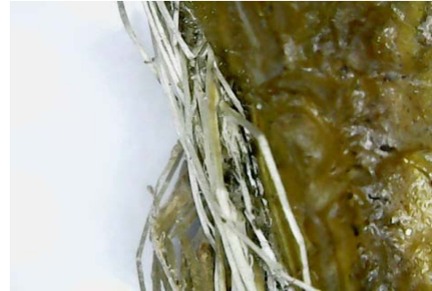
Fig. 10: Microscopic image-tear failure edge (90° fibers)
