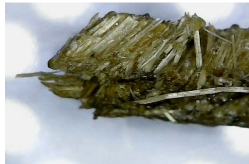
Fig. 7: Microscopic image-tensile failure edge (90° fibers)
