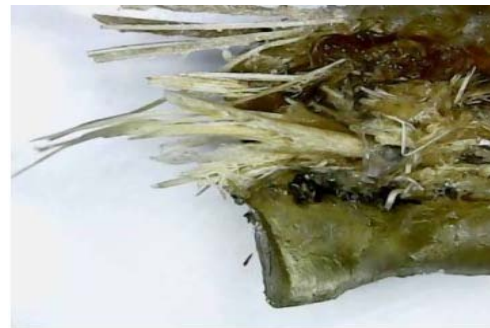
Fig. 6: Microscopic image-tensile failure edge (0° fibers)
