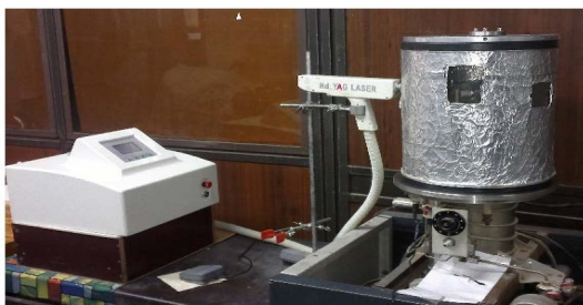
Fig. 1: PLD set up using Nd: YAG
