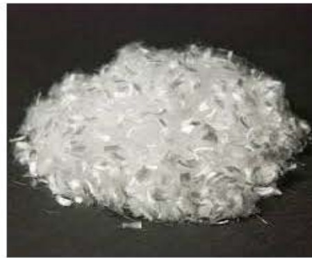
Fig. 2: Fibrillated polypropylene fibers used in present work
