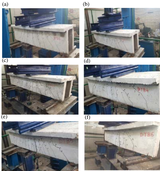
Fig. 6: a-f) Double tee beams with PPF after test
