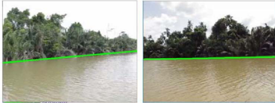
Fig. 3: Simulation results of shoreline detection constrained Hough transform
